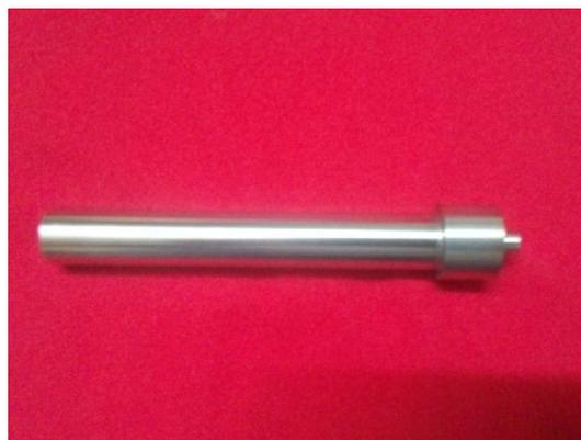
**Fig. 6 Friction Stir Welding Tool**
