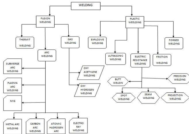
Fig. 1 Types of Welding Process
